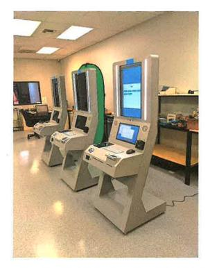
Approximately 250 lbs - Standard 110V AC Power provided by a single C14 power input connection (bottom rear) with both surge protection and a UPS built in
